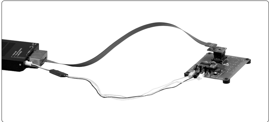
Figure 3.10 Connecting the M38000TL2-FPD (when using RLSS/RLFS type emulator MCU)
